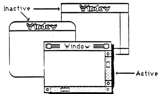
The Window Manager's main function is to keep track of overlapping windows. You can draw any window without running over onto windows in front of it. You can move windows to different places on the screen, change their plane (front-to-back order), or change their size, all without concern for how the various windows overlap. The Window Manager keeps track of any newly exposed areas and provides a convenient mechanism for you to ensure that they are properly redrawn.
