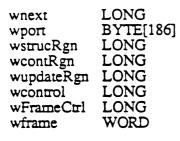
Pointer to the next window in the window list. Window's port. Returned window pointers return a pointer to here. Handle of window's entire region, the frame plus content. Handle of window's content region. Handle of region that is the part of the content that needs redrawing. Handle of application's first control in content region. Handle of frame's first control. Bit vector that describes window.
