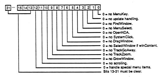
It is important that bits 13-31 be clear. In fact, TaskMaster will return an error if they are not. The bits are for future features which will continue to run with predated applications because bits 13-31 will mask off the new, unknown to current applications, features.
