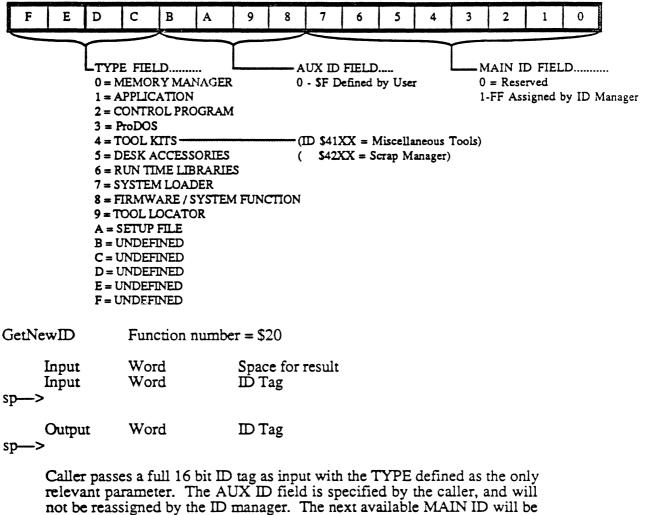
not be reassigned by the ID manager. The next available MAIN ID will be concatenated to the TYPE and AUX ID fields, and the resulting ID Tag will be returned to the caller. Note that the TYPE field must be non zero. Note that only 255 ID tags can be assigned for any TYPE ID. If an ID cannot be assigned because all the ID tags for that TYPE have been assigned, then an error will be returned indicating that the ID is not available.
