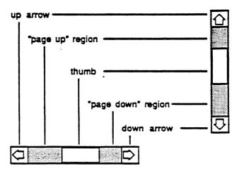
The parts of the scroll bars can be generalized into three regions; arrows, paging, and thumb (or thumber). The arrows scroll data a line at a time, paging regions scroll a "page" at a time, and the thumb can be dragged to any position within the scroll area. Although they may seem to behave like individual controls, these are all parts of a single control, the scroll bar type of dial. You can define other dials of any shape or complexity for yourself if your application needs them.
