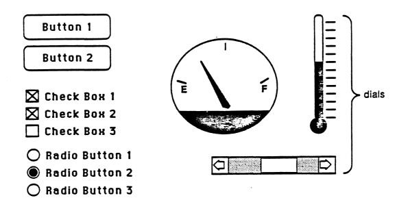
Certain standard types of controls are predefined for you. Your application can easily use controls of these standard types, and can also define its own "custom" control types. The predefined control types are the following:
