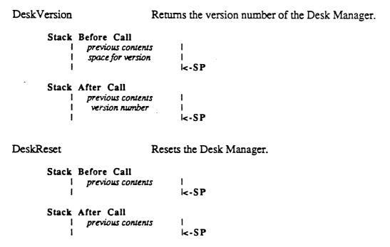
This call should not be made by an application. It is made by the Reset handler built into ROM. It is only called when a user presses CONTROL-RESET.
